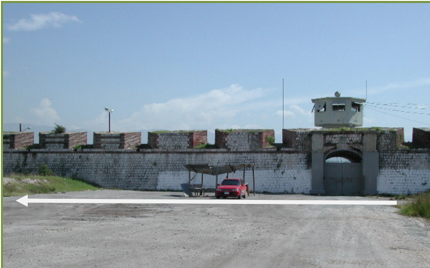
PLATE 2 Sand covering entire width of road that leads to the Fort Augustus prison. The arrow indicates the run-up distance of approximately 90m.
