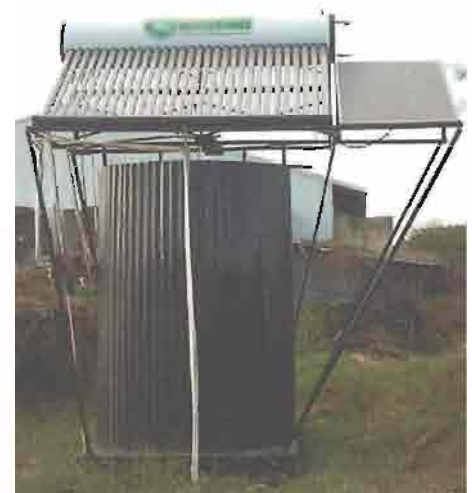
The DBJ supported the development of the 'solar hydronic brooder' that utilises solar energy as its heat source.
